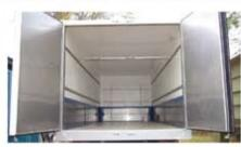
Hold bars with stainless steel side and wall plates.
